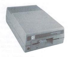
drive needs a unique number. The most basic drives, the 1541 and 1571, range up to 11. These either have small DIP switches on the back to select the number (new style) or must be modified internally (old style) to make the change. So, you can use this program to ensure that each drive on the chain shows up once if you're short a drive, you should recheck all of your cabling, power, and device number selection and then try again.
